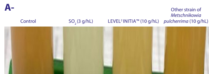
Chardonnay must (France) after pressing. Comparison of different solutions of protection against oxydation.
